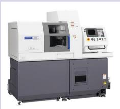
Citizen L20 type X screw machine with live front and back live tooling. Full C-axis front and back. with full length barloader and 2000 psi coolant. Can machine complex parts completely unattended.
