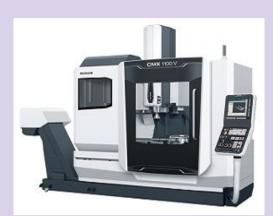
DMG Mori CMX 1100V 2018 X 43" Y 22" Z 20" travels 15000 RPM 12.1 HP spindle Factory installed DDR 4TH AXIS
